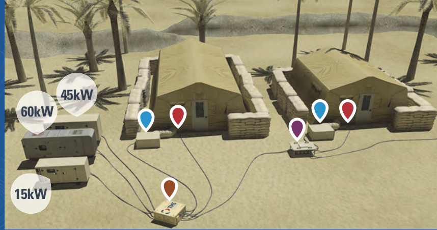
POWER MANAGEMENT MODULE POWER FLOW EXAMPLE
